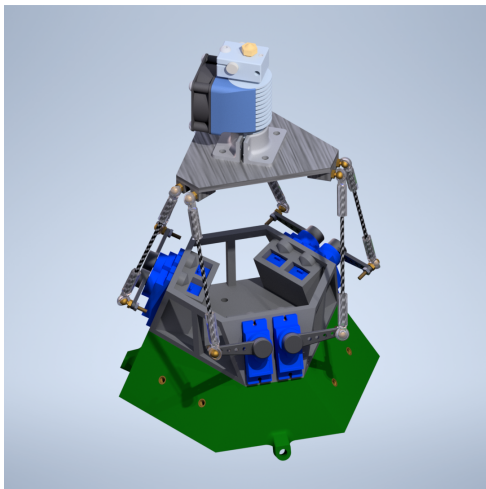
Figure 4.4: Previous Acrobat version rotary Stewart platform
